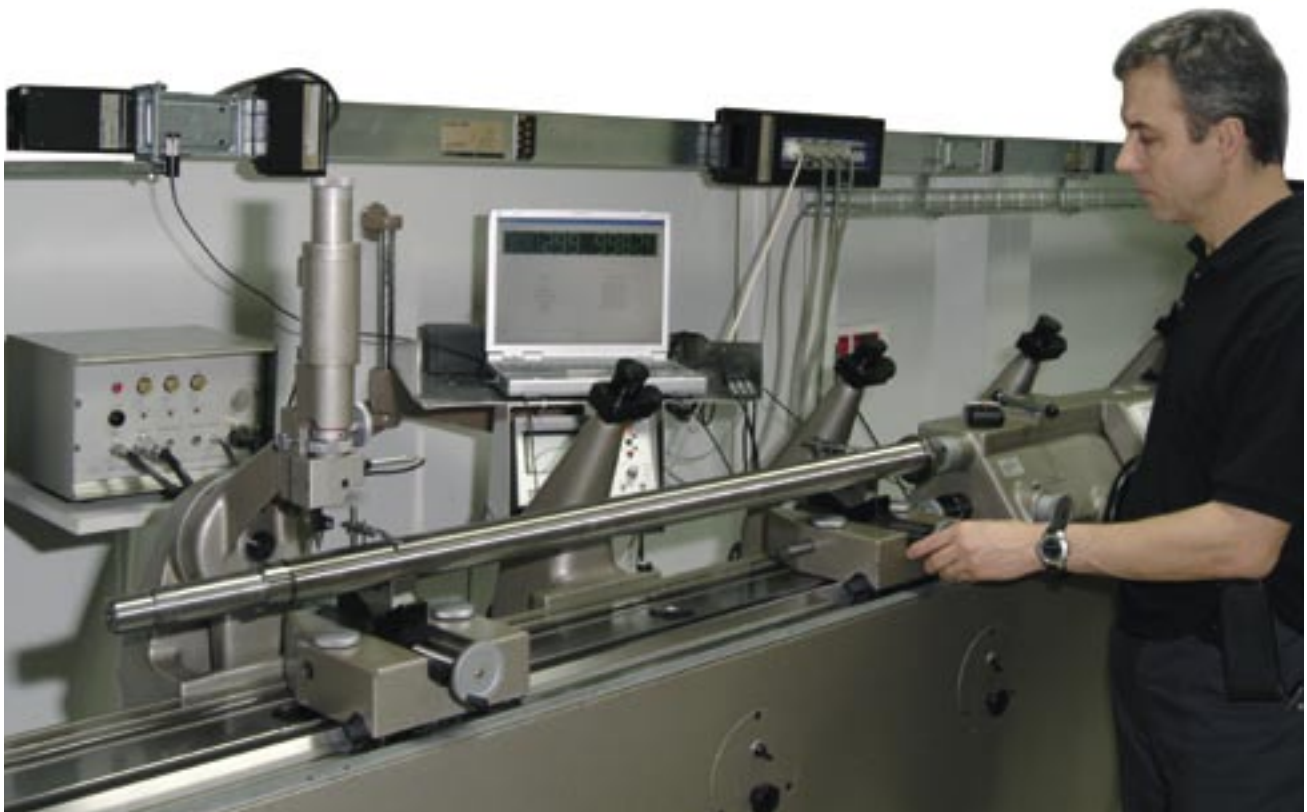
Lead error control interferometric test bench
